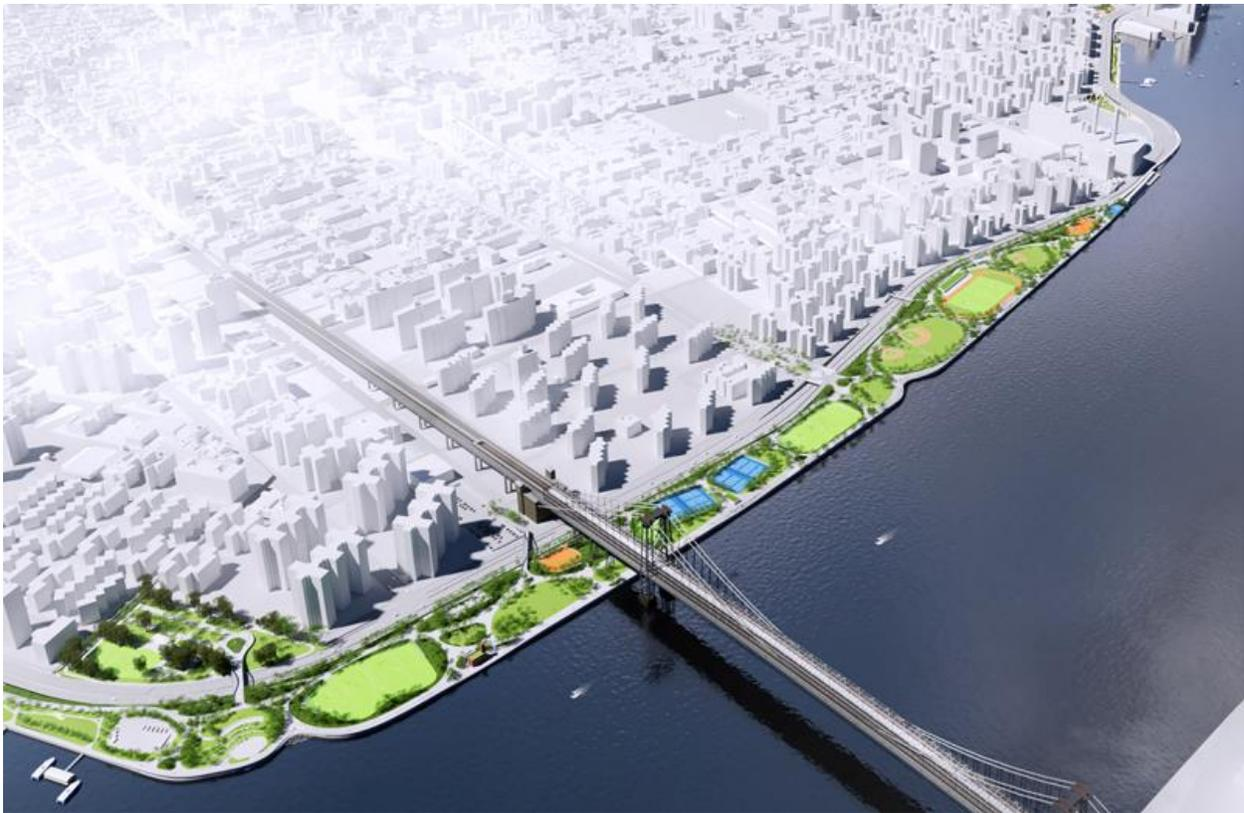
**The East Side Coastal Resiliency project uses a series of berms, flood walls, flood gates and raised parklands to create a continuous 2.4-mile barrier to protect 110,000 residents of the Lower East Side in Manhattan from future coastal and tidal flooding**
